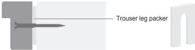
Note: The lateral force at the bottom hinge position can compress packings and metal studs causing the leading edge to drop. Before installing, ensure that studs are secure and fillings are dry.
